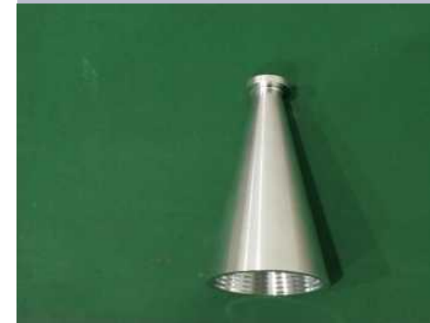
Figure 8. 7 mm shaped corrugated horn feed model and physical processing diagram
