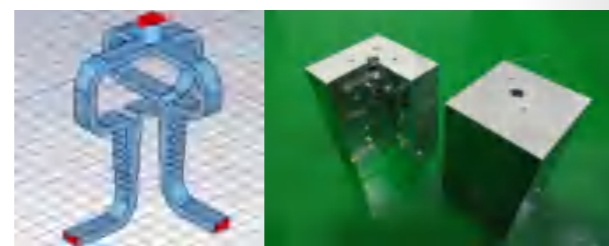
Figure 7. 7 mm OMT model and physical processing diagram
